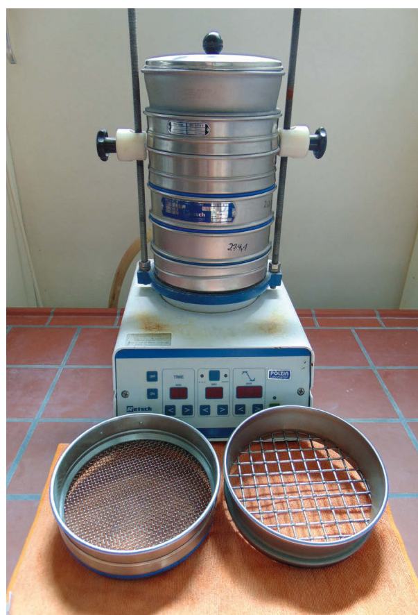
Fig. 6.5. Sieving machine as used for quantifying fecal particle sizes of herbivores. Photo: J. Hummel.
